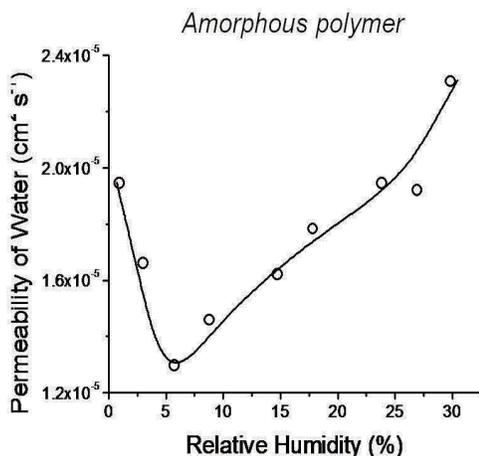
The figure to the left shows the permeability of water vapor in the polymer Eudragit E-100 as a function of relative humidity (RH). With sorbed water acting as a plasticizer, the common expectation is that permeability ought to increase as the amount of water present increases. This is indeed the case, with the notable exception of the first portion of the curve. When water is present at very low levels, it depresses permeability before greater concentrations begin to increase it.
