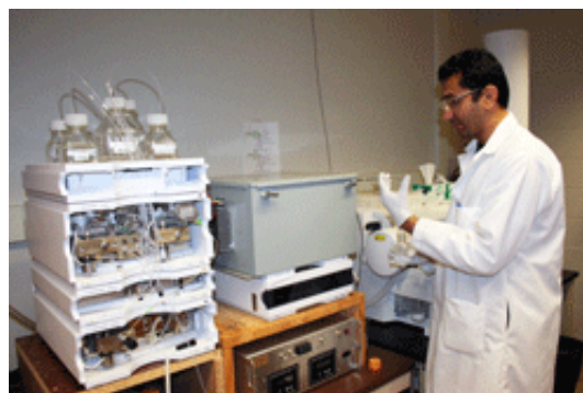
Jainik Panchal injects a sample into the LC-MS to characterize the mass of a protein molecule
